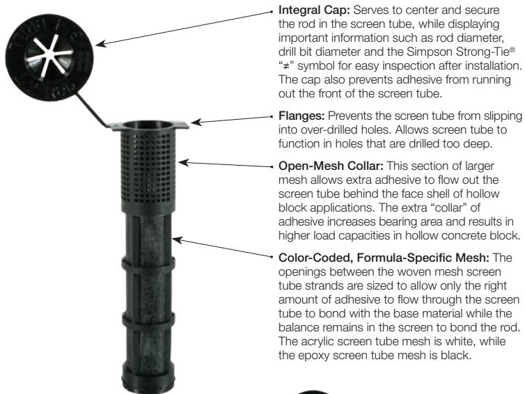
Epoxy Adhesive Screen Tube (mesh is black)
